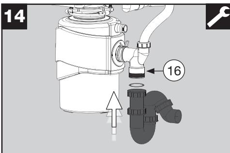
Connect your odour trap/siphon (not included in scope of delivery) to the lower outlet of the outlet elbow pipe (16) and to your building waste water connection.
