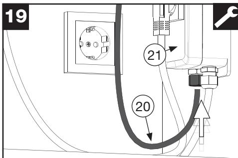
Connect the other end of the air hose (20) to the switch box (21) and secure the hose with the hose nut as described in Step 18.
