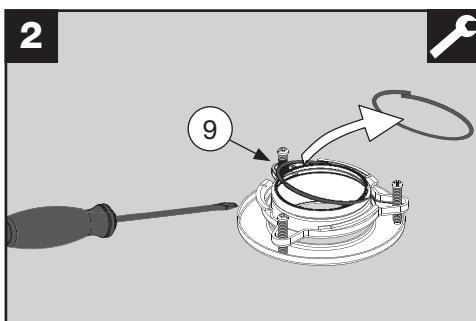
Use a long slotted-head screwdriver to lever out the circlip (9) and put it to one side.
