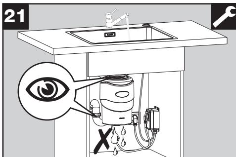
Put the disposer into operation as described in the following chapter, Initial Start-Up. To finish off, check all hose and pipe connections and the sink drain for any leaks.
