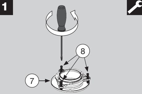
Loosen the three screws (8) on the holding ring (7) but do not undo them completely.
