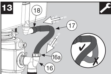
Push the overflow adapter (18) onto your sink overflow (until it locks into position).
