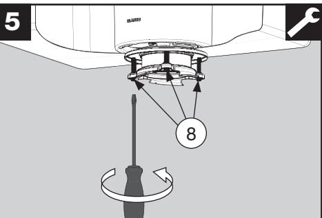
Tighten the three screws in the holding ring (8) evenly.
