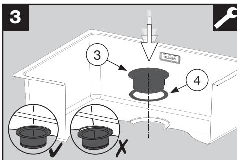
Attach the sink flange (3) together with the rubber seal on top (4) into the sink drain opening. Ensure you position it in the centre.
