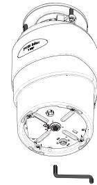
4. Carefully remove the foreign object from the grinding chamber. You might like to use tools such as a pair of pliers or a screwdriver with a long handle.
