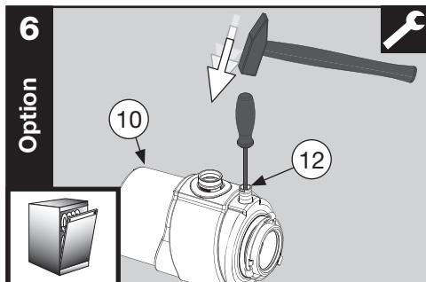
Optional (only use if the dishwasher outlet is to be connected to the disposer):
