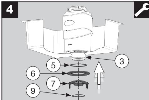
Push the lower seal (5), the retaining ring (6) and the holding ring (7) onto the sink flange from below and press the circlip (9) into the groove in the sink flange (3).
